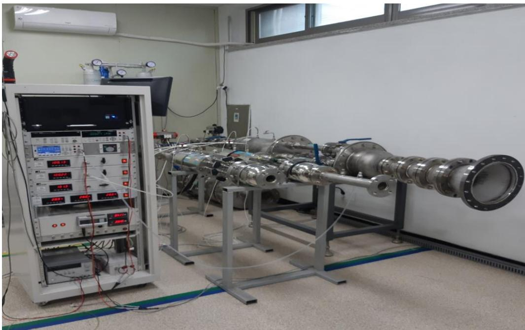
CORIOLIS MASS FLOW METER (Liquid)
