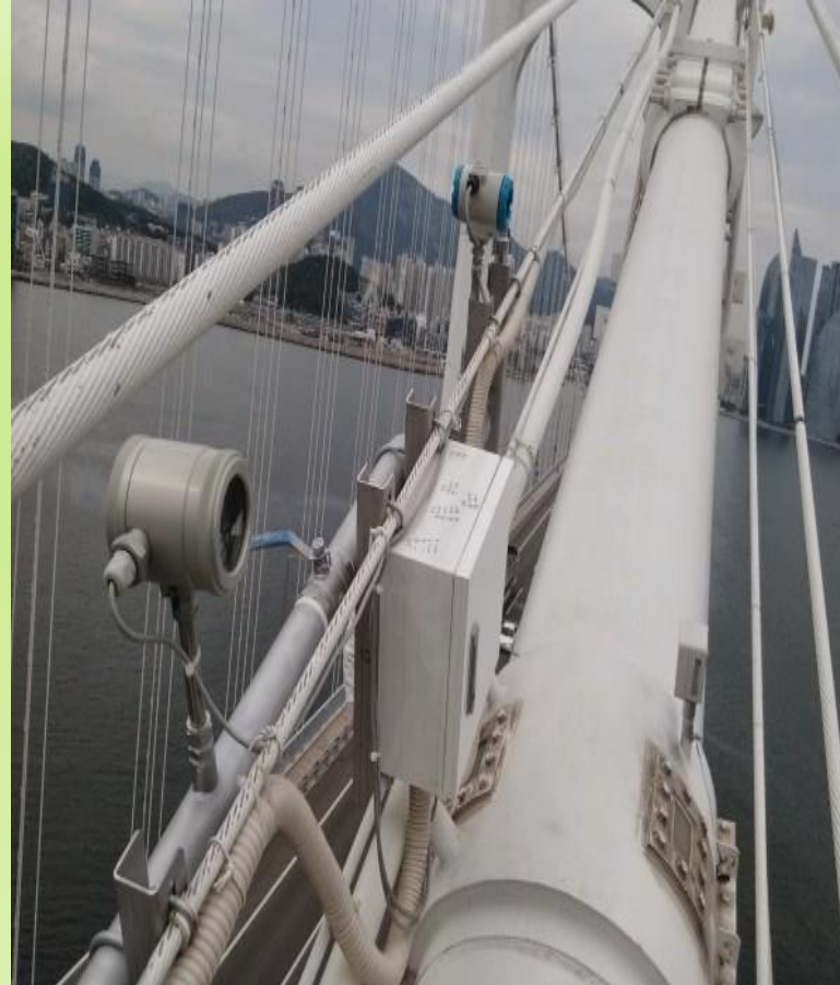
Busan Gwangan Bridge & Yeongjong Bridge Thermal flow meter for cable air Insertion valve type ~ 20 units delivered
